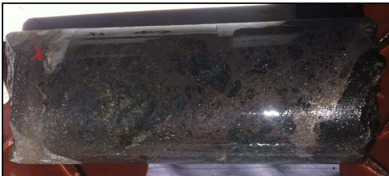
Figure 2: Sulphide (pyrrhotite) breccia 10 cm thick with minor copper (chalcopyrite) mineralisation hosted by altered meta-sediments in 12AMD0018 (depth 260.15 metres)
