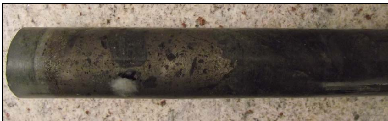
Figure 4: Sulphide (pyrrhotite) breccia 15 cm thick with minor copper (chalcopyrite) mineralisation hosted by altered meta-sediments in 12AMD0021 (depth 311.0 metres)
