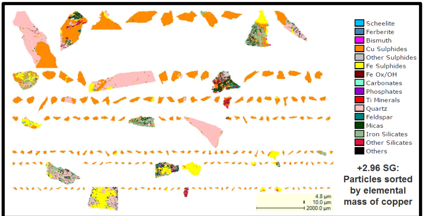
Figure 4: Calibre metallurgical test work QEMSCAN® image of particles sorted by the elemental mass of copper showing coarse grained and well liberated nature of copper sulphides (chalcopyrite) (NB: grind size 100% passing 3.35mm)
