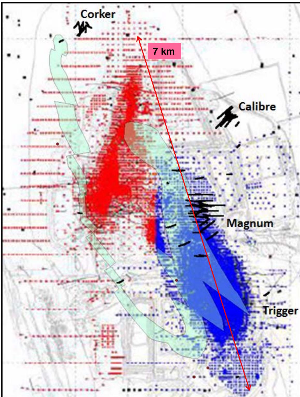
**Figure 8:** Telfer Dome (Moorhead, 2014) superimposed at the same scale on the Magnum Dome (defined by transparent green interpreted Magnum Gabbro) showing Telfer ore grade control drilling (dense masses of blue and red dots) and Magnum Dome Diamond and RC drillholes (black lines) (2km dashed grid)
