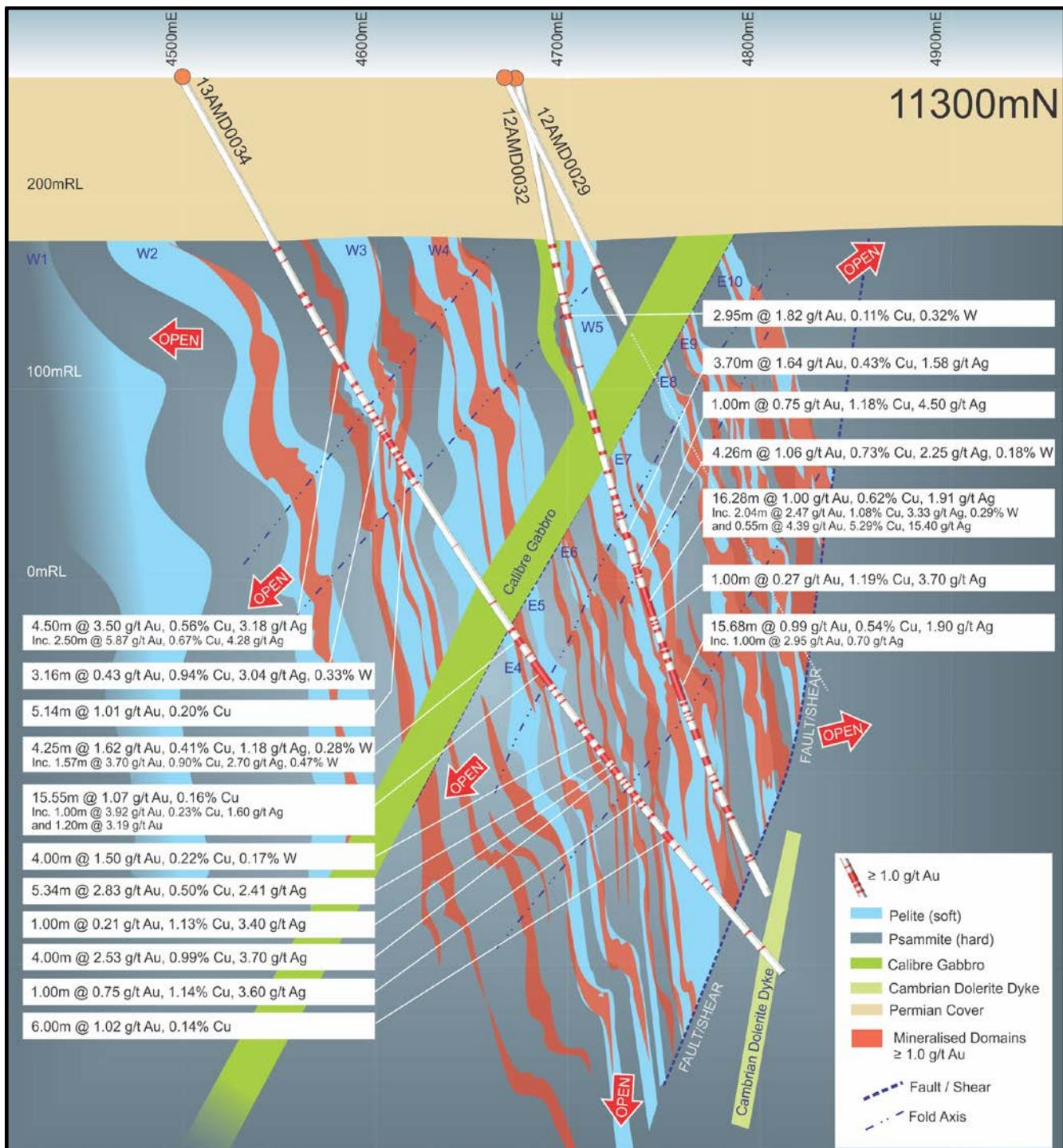
**Figure 3: Calibre Deposit 11300 North interpreted (schematic) cross-section showing folded interbedded (hard) quartzite and (soft) pelite metasedimentary packages with  $\geq 1 \text{ g/t gold}$  mineralisation generally internal to or on the margins of the pelite dominated units (100m grid)**
