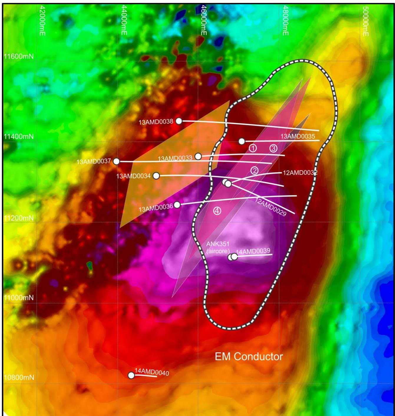
**Figure 7:** Calibre prospect total (ground) magnetic intensity reduced to the magnetic pole with a northeast sun shading showing location (projected vertically to surface) of the FLEM Z-component gradient (Channel 16) electromagnetic conductivity anomaly, drillholes and DHEM conductivity plate models (numbered 1 to 4).
