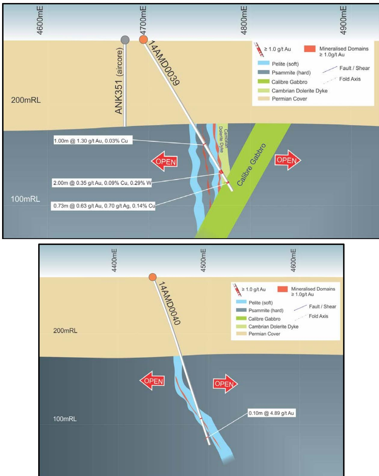
**Figures 6a-b: Calibre Deposit 11120 North and 10820 North interpreted (schematic) cross-section showing folded interbedded (hard) quartzite and (soft) pelite metasedimentary packages with  $\geq 1 \text{ g/t}$  gold mineralisation generally internal to or on the margins of the pelite dominated units (100m grid)**
