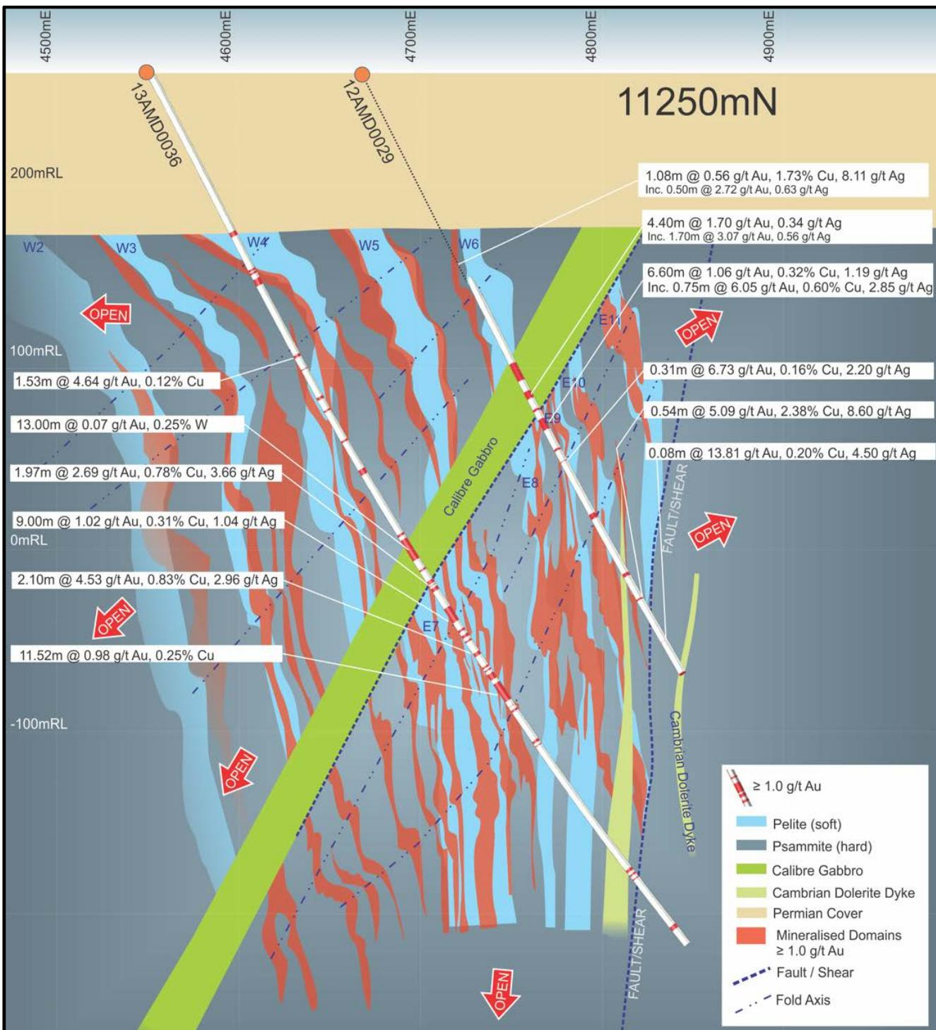
**Figure 2: Calibre Deposit 11250 North interpreted (schematic) cross-section showing folded interbedded (hard) quartzite and (soft) pelite metasedimentary packages with  $\geq 1$  g/t gold mineralisation generally internal to or on the margins of the pelite dominated units (100m grid)**
