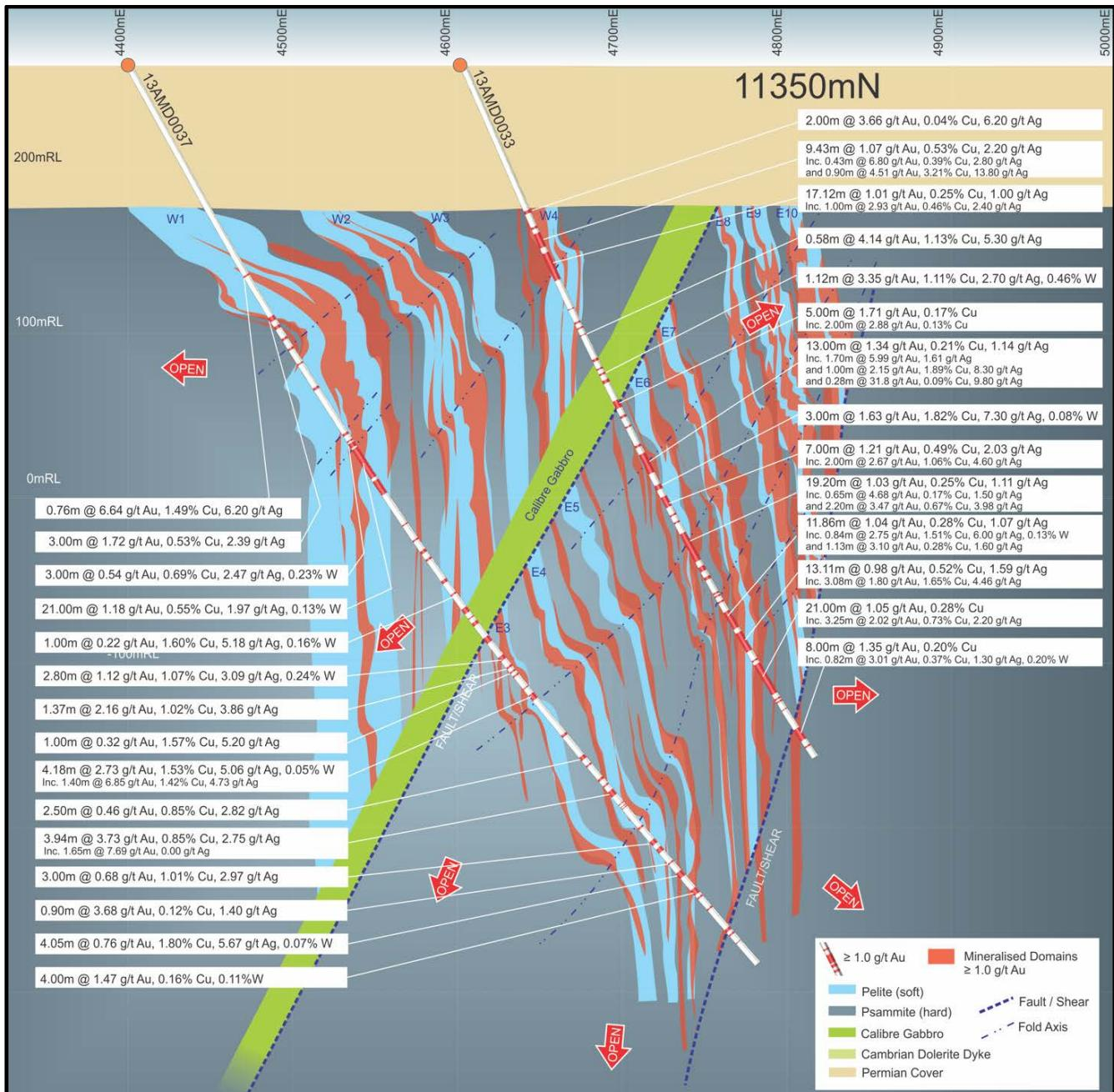
**Figure 1: Calibre Deposit 11350 North interpreted (schematic) cross-section showing folded interbedded (hard) quartzite and (soft) pelite metasedimentary packages with  $\geq 1 \text{ g/t}$  gold mineralisation generally internal to or on the margins of the pelite dominated units (100m grid)**
