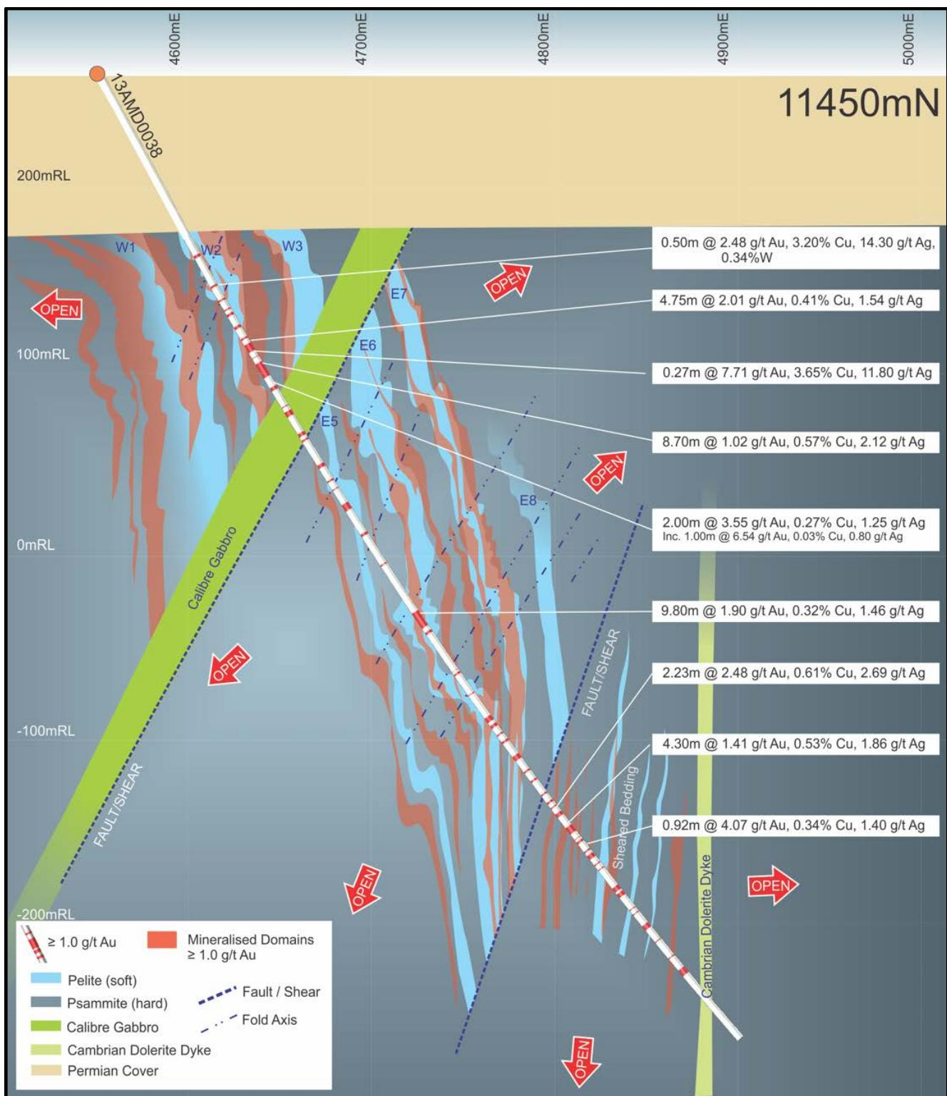
**Figure 5: Calibre Deposit 11450 North interpreted (schematic) cross-section showing folded interbedded (hard) quartzite and (soft) pelite metasedimentary packages with  $\geq 1 \text{ g/t}$  gold mineralisation generally internal to or on the margins of the pelite dominated units (100m grid)**
