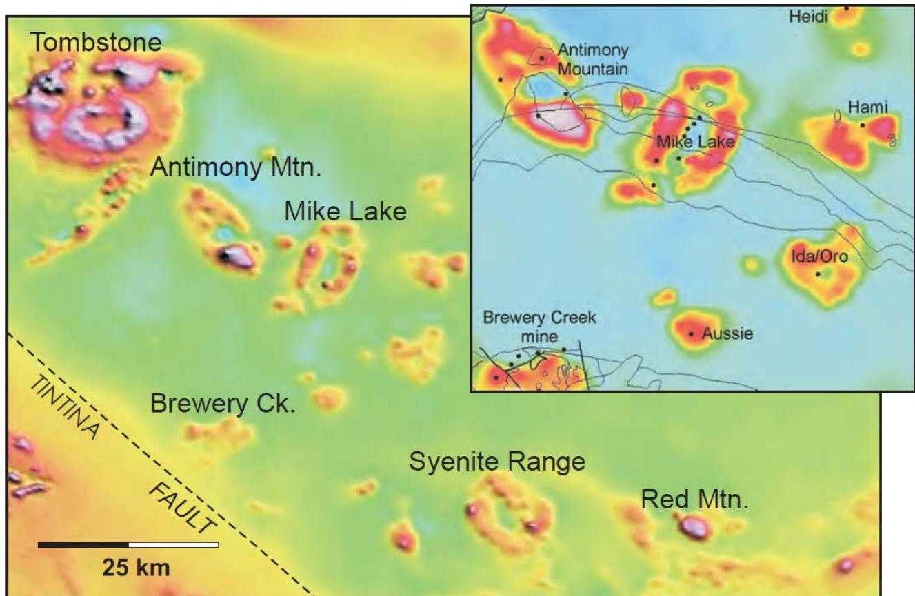
**Figure 9:** Aeromagnetic image for a portion of the TGP showing low magnetic response plutons, many of which can be identified by their magnetic pyrrhotite bearing aureoles (Scale Bar 25km). Inset shows detailed magnetic features in the TGP's Mike Lake area, with the black dots indicating mineral occurrences (Hart et al., 2007). Note similarities to Citadel Project in Figure 9 below.
