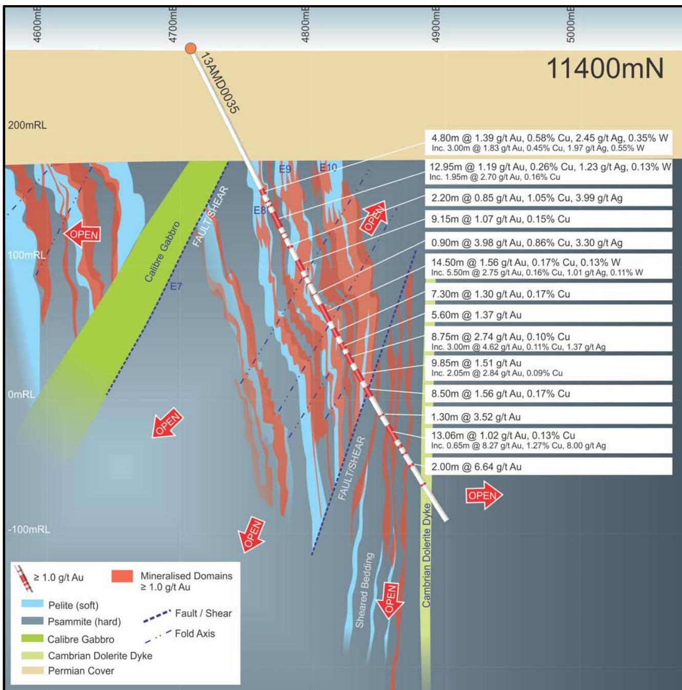
**Figure 4: Calibre Deposit 11400 North interpreted (schematic) cross-section showing folded interbedded (hard) quartzite and (soft) pelite metasedimentary packages with  $\geq 1$  g/t gold mineralisation generally internal to or on the margins of the pelite dominated units (100m grid)**
