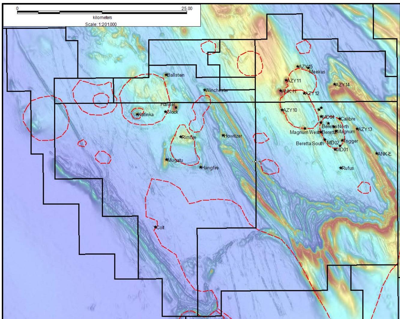
**Figure 10: Aeromagnetic image for the Company's 1,595km<sup>2</sup> Citadel Project (tenements outlined in black) showing low magnetic response plutons, many of which can be identified by their magnetic pyrrhotite bearing aureoles, and deposit and prospect locations (Scale Bar 25km). Interpreted plutons red dashed lines (NB: Drilling and gravity data also assisted with the granite interpretation). Note similarities to TGP in Figure 8 above.**
