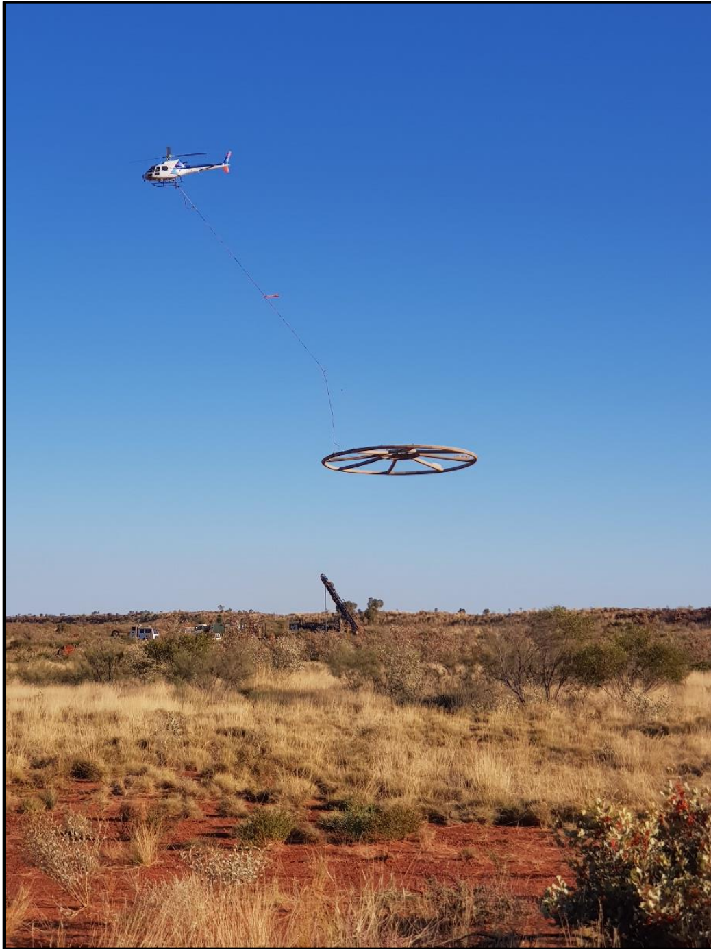
Figure 5: New Resolution Geophysics (NRG™) Xcite™ helicopter-borne time-domain electromagnetic loop passing by a reverse circulation drill rig at Antipa's Minyari Dome area.
