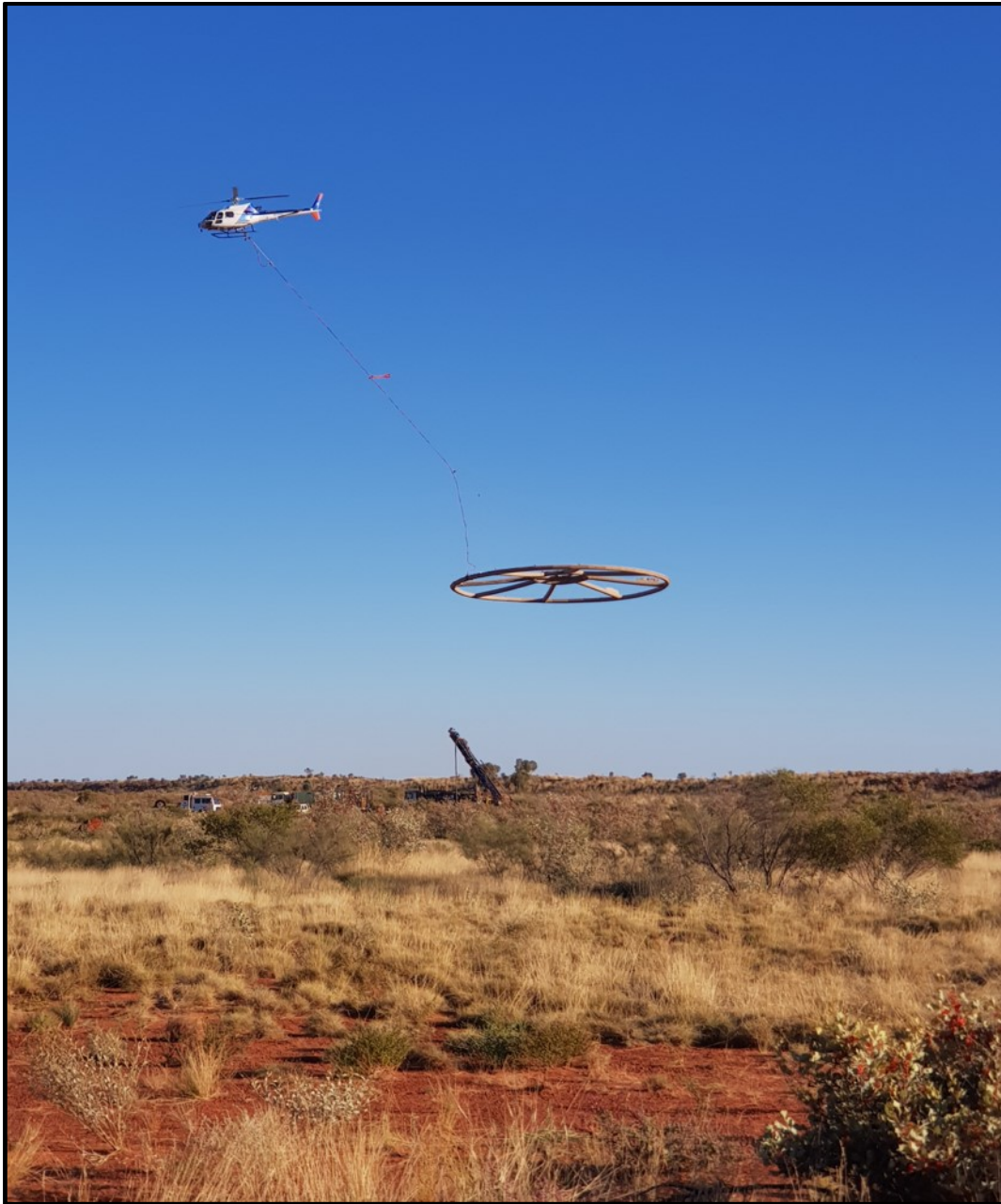
Figure 4: New Resolution Geophysics (NRG™) high precision Xcite™ helicopter-borne time-domain electromagnetic (HTDEM) system in action during the 2018 AEM survey.
