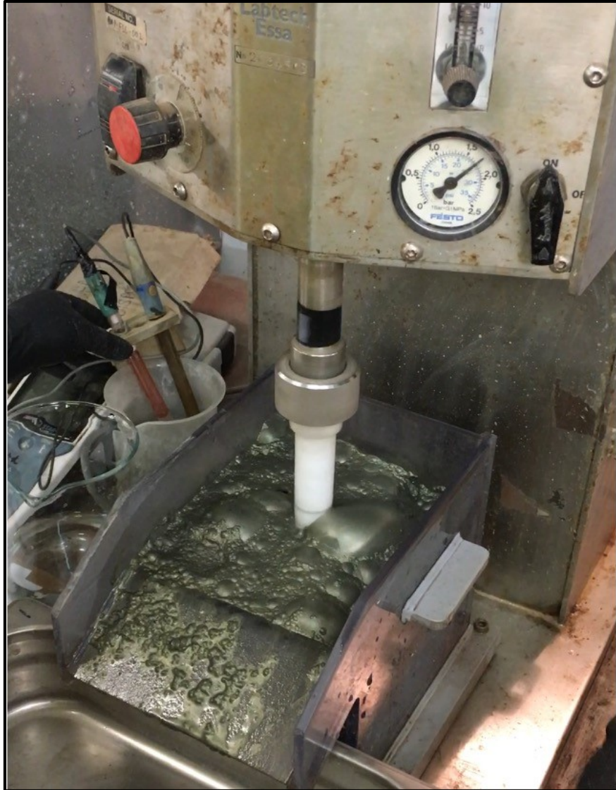
Minyari Deposit metallurgical test-work copper sulphide float
