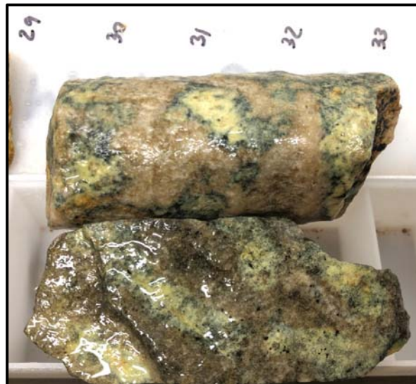
Figure 2: GAIP07 area air core drill hole 20MYA0017 sample from 30m showing “digestive”/replacive brecciation resulting from intrusion related intense hydrothermal alteration, with possible disseminated ex-sulphide “spotting”
