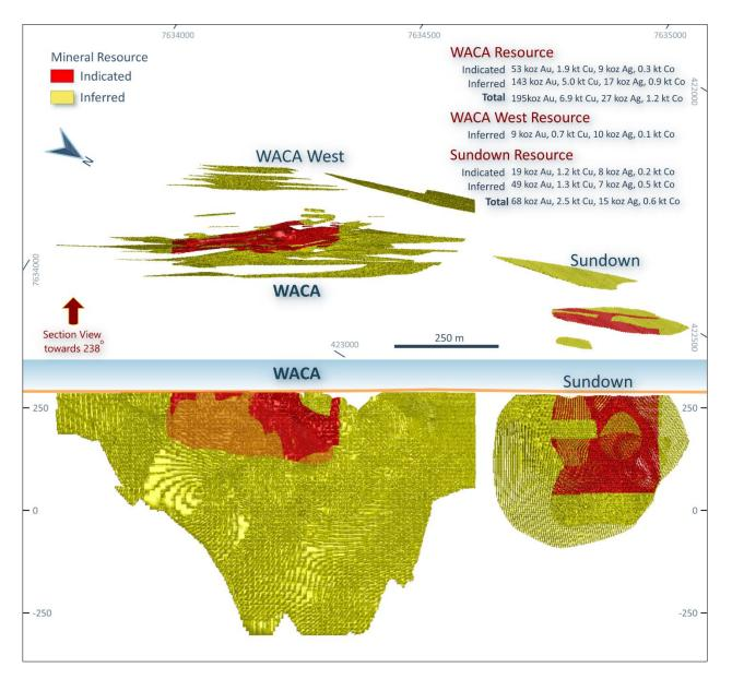
**Figure 7: WACA, WACA West and Sundown deposits Plan and Long Projection views showing distribution of gold-coppersilver-cobalt Indicated and Inferred Mineral Resource.** NB: Regional GDA2020 / MGA Zone 51 co-ordinates, with 500m plan grid and 250m vertical grid, main Long Projection looking horizontally toward Local Grid bearing 270° (or 238° MGA Zone 51).
