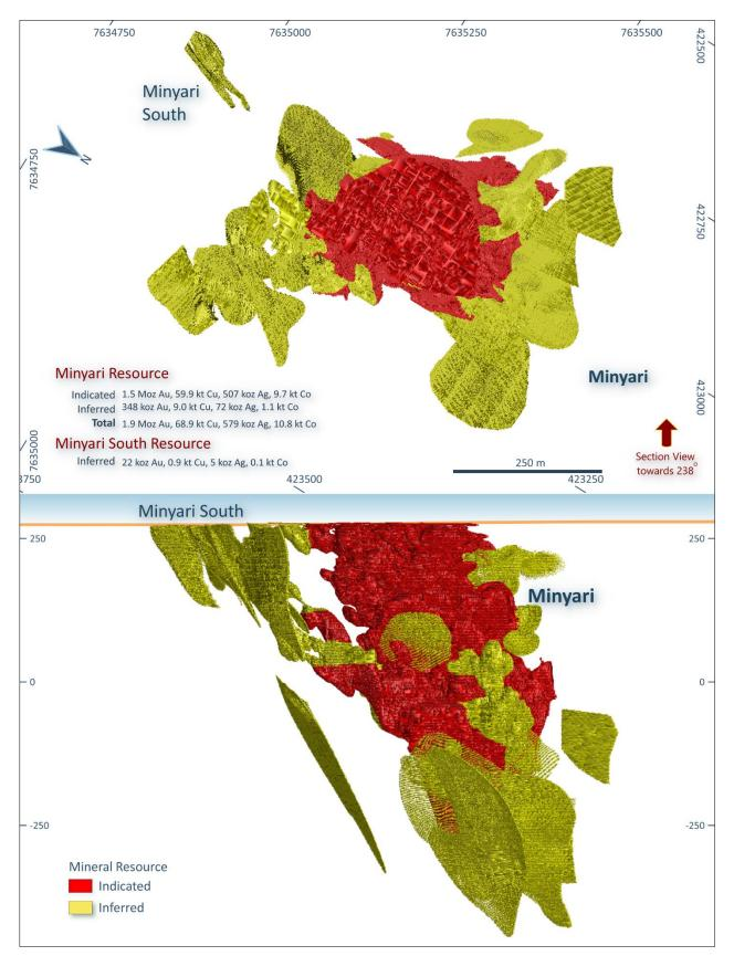
**Figure 5: Minyari and Minyari South deposits Plan and Long Projection views showing distribution of gold-copper-silver-cobalt Indicated and Inferred Mineral Resource.** NB: Regional GDA2020 / MGA Zone 51 co-ordinates, with 250m plan grid and 250m vertical grid, main Long Projection looking horizontally toward Local Grid bearing 270° (or 238° MGA Zone 51).
