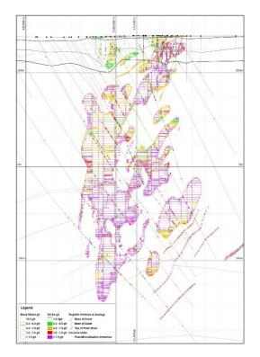
Figure 10: Minyari deposit cross-section Local Grid 100,700mN, looking Local Grid north (MGA Zone 51 Bearing 328°), showing estimated gold grades in Mineral Resource block model and drill holes showing gold grades. The grid squares represent 200m.
