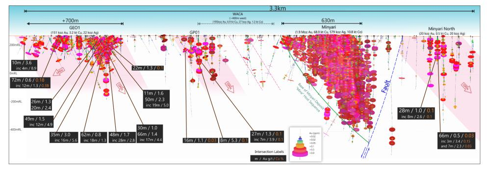
Figure 9: Long Section from GEO-01 to Minyari North including Minyari and GP01 showing gold drill intercepts and interpreted key features including multiple zones of plunging goldcopper mineralisation. Note the highly prospective 3.3km trend which extends to 4.6km including the Judes copper-silver-gold deposit. NB: 200m elevation (RL), looking toward Local Grid 270° (or 238° MGA Zone 51 Grid).
