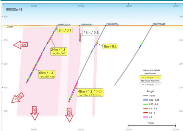
Figure 1: GEO-01 stacked cross-section showing first-pass broad spaced RC gold-copper drill intercepts original four metre composite samples.
